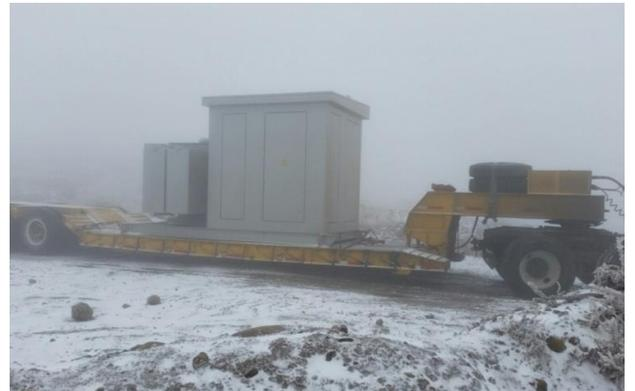
The main electrical transformer for the LSST summit site was delivered to enable connection to the main power grid and to move away from the need to use local generator power.
