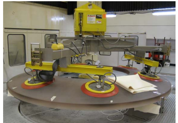
The secondary mirror (M2) being lowered onto a support body to begin measurement of the optical surface.
