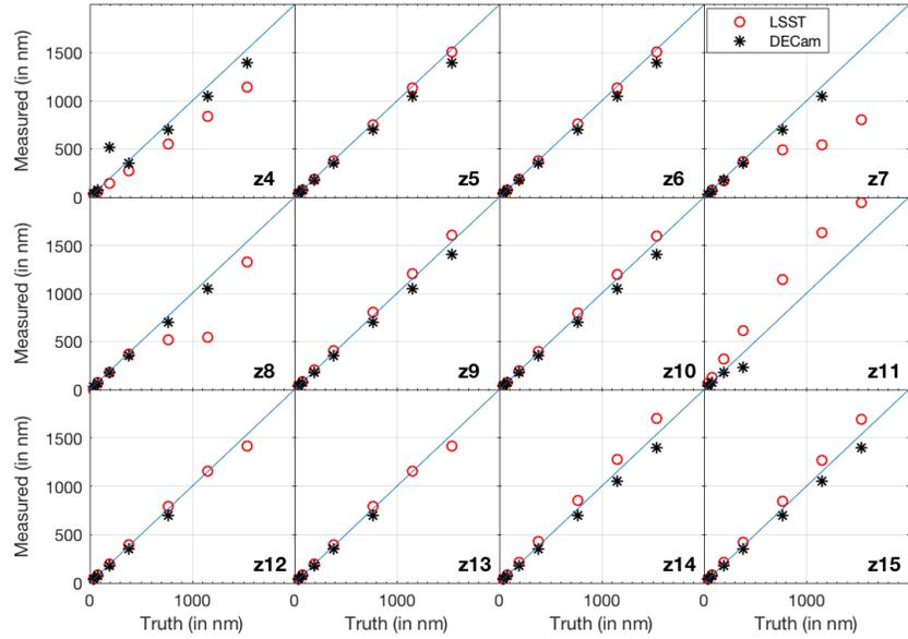
Figure 7. Comparison of wavefront recovery results using images simulated with the DECam forward-modeling code. The blue diagonal lines with slope of unit are for reference.
