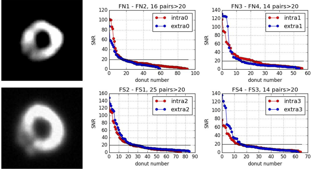
Figure 1. Left: An intra-focal image (top) on wavefront sensor FN1 and an extra-focal image (bottom) on wavefront sensor FN2. Right: SNR distributions on the pairs of wavefront sensors. The plot titles show the sensor names and the number of image pairs where both images have SNR >20. These examples are with the telescope in the open-loop mode.
