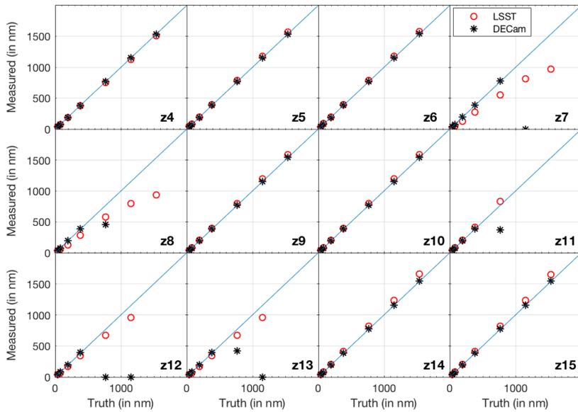
Figure 8. Comparisons of wavefront recovery results using ZEMAX-simulated images. The blue diagonal lines with slope of unit are for reference.
