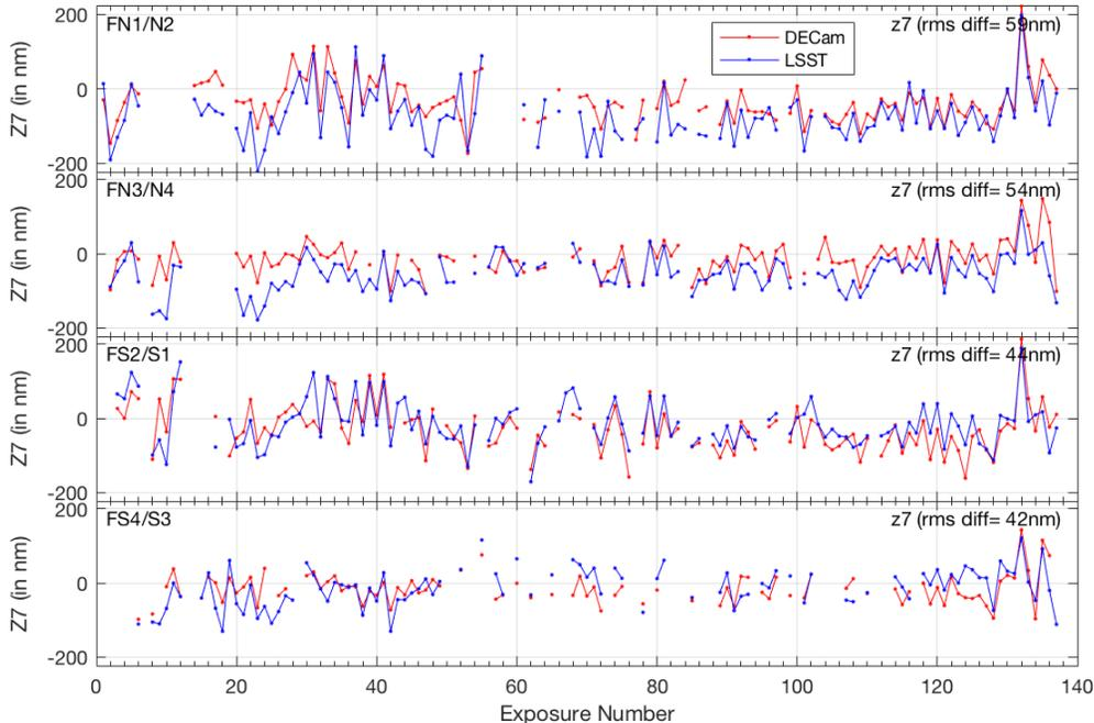
Figure 5. Variations of coma-y ( $Z7$ ) through a typical DECcam observing night, as measured by the DECcam (red) and LSST (blue) algorithms. The four panels are for the four pairs of wavefront sensors. The RMS differences between the measurements by the two algorithms are shown in the upper right corner of each panel.
