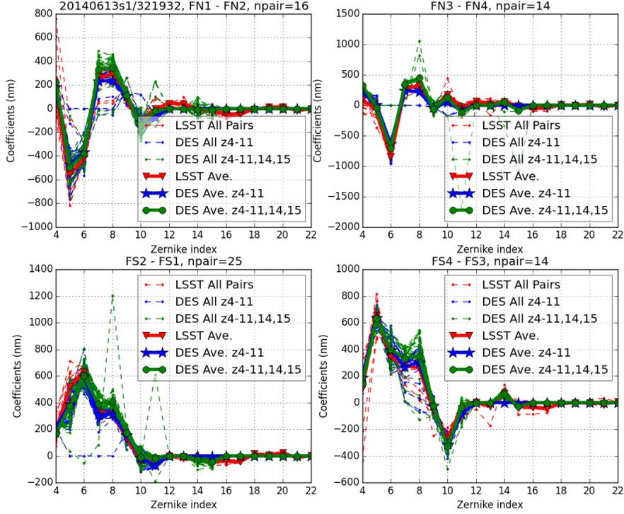
Figure 2. Comparison of Zernike coefficients using one exposure from the open-loop wavefront images.
