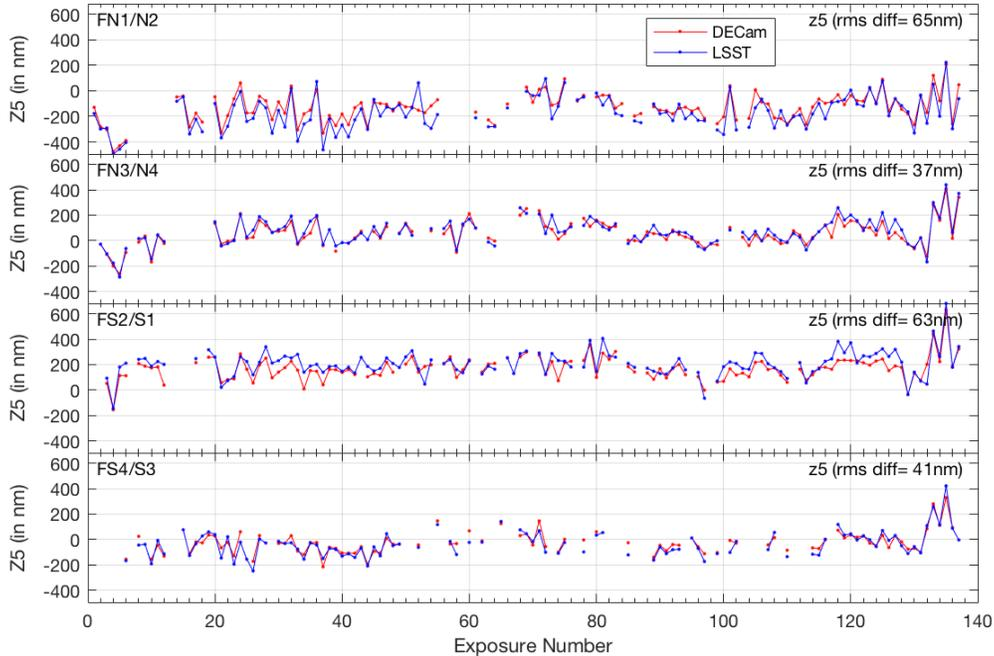
Figure 4. Variations of  $45^\circ$  astigmatism ( $Z_5$ ) through a typical DECcam observing night, as measured by the DECcam (red) and LSST (blue) algorithms. The four panels are for the four pairs of wavefront sensors. The RMS differences between the measurements by the two algorithms are shown in the upper right corner of each panel.
