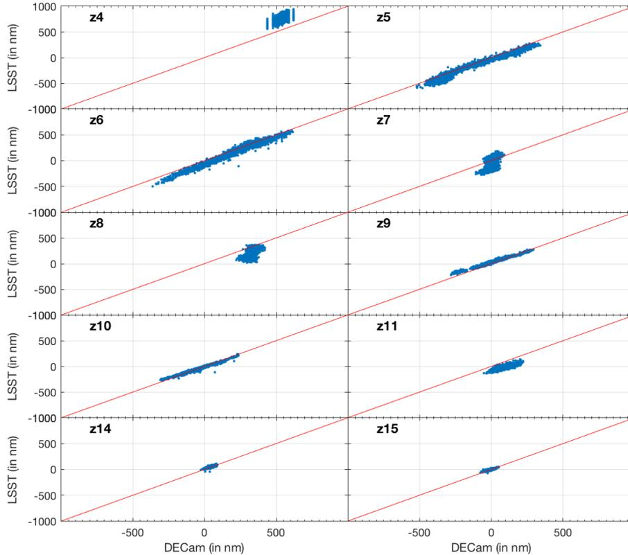
Figure 6. Scatter plots of DECam results vs. LSST by Zernike. The data used are out-of-focus science sensor data with the camera hexapod pistoned by  $\pm 1.5$ mm. The red diagonal lines with slope of unit are for reference.
