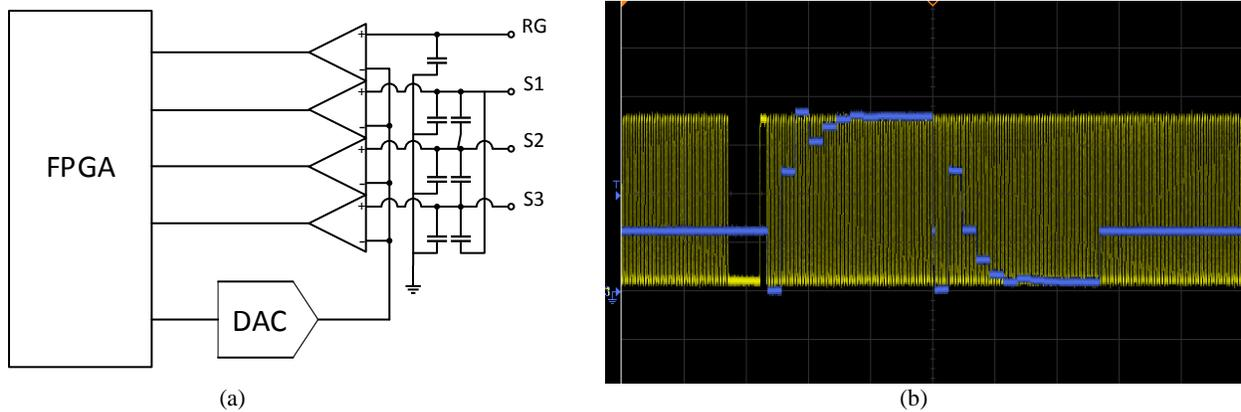
Figure 5. (a) The schematic for Serial clock and Reset Gate clock detection. (b) Clock level sweep in the binary search method. The yellow line is the serial clock signal, while the blue line is the sweeping signal.
