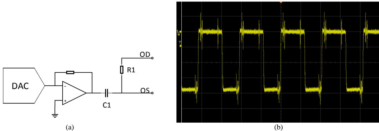
Figure 4. (a) Video generation diagram. (b) Output video signal generated by the CCD emulator.
