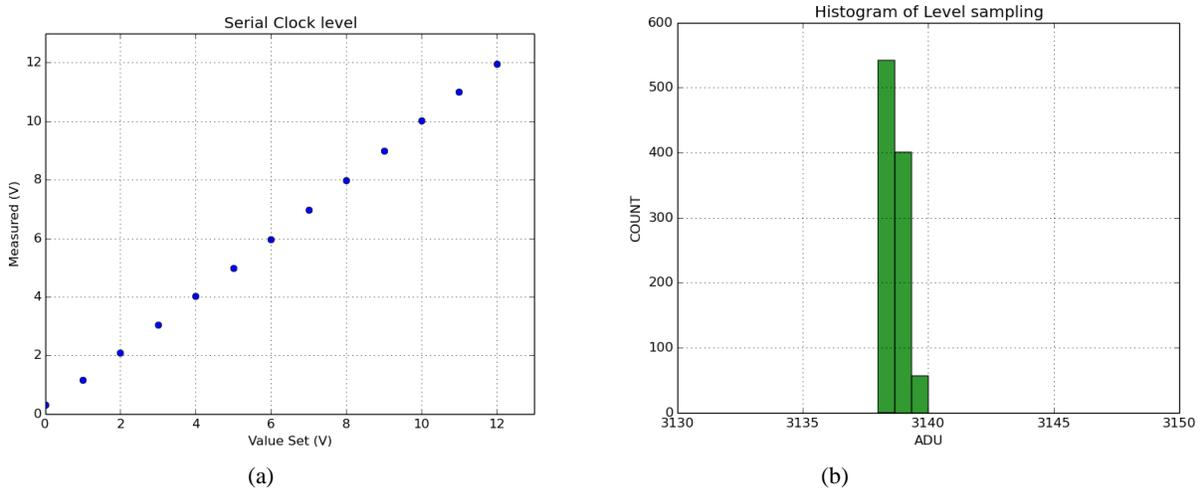
Figure 8. Performance of clock level sweeping. (a) Linearity, (b) Histogram.
