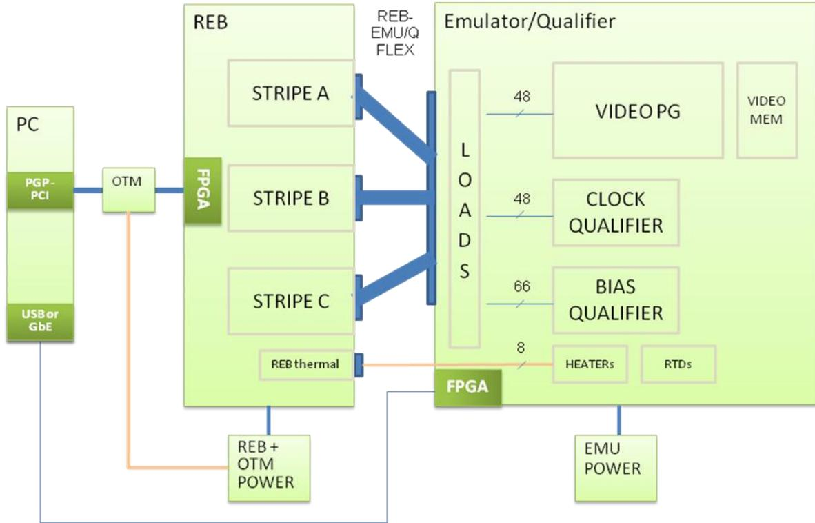
Figure 1, Block diagram of REB test station
