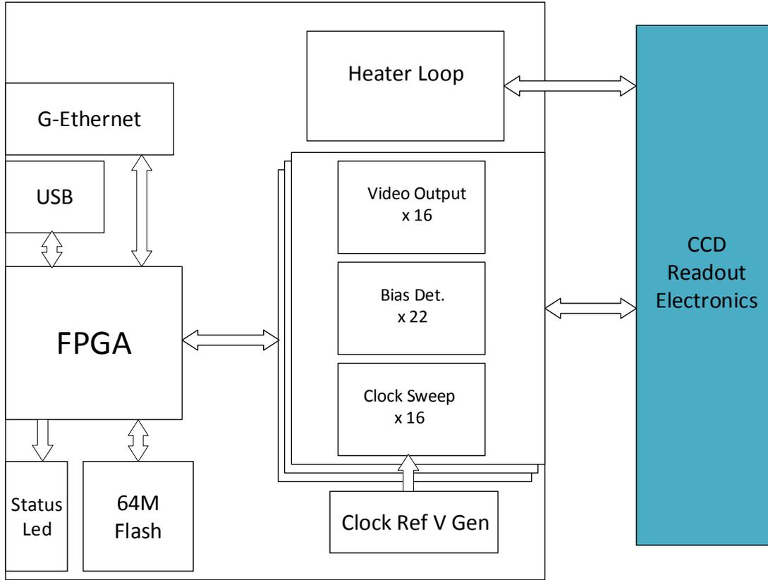
Figure 3. Block diagram of the CCD emulator
