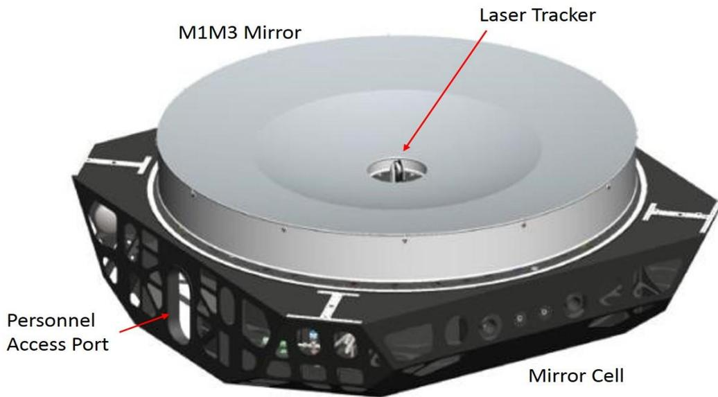
Figure 6: Integrated M1M3 mirror cell assembly.
