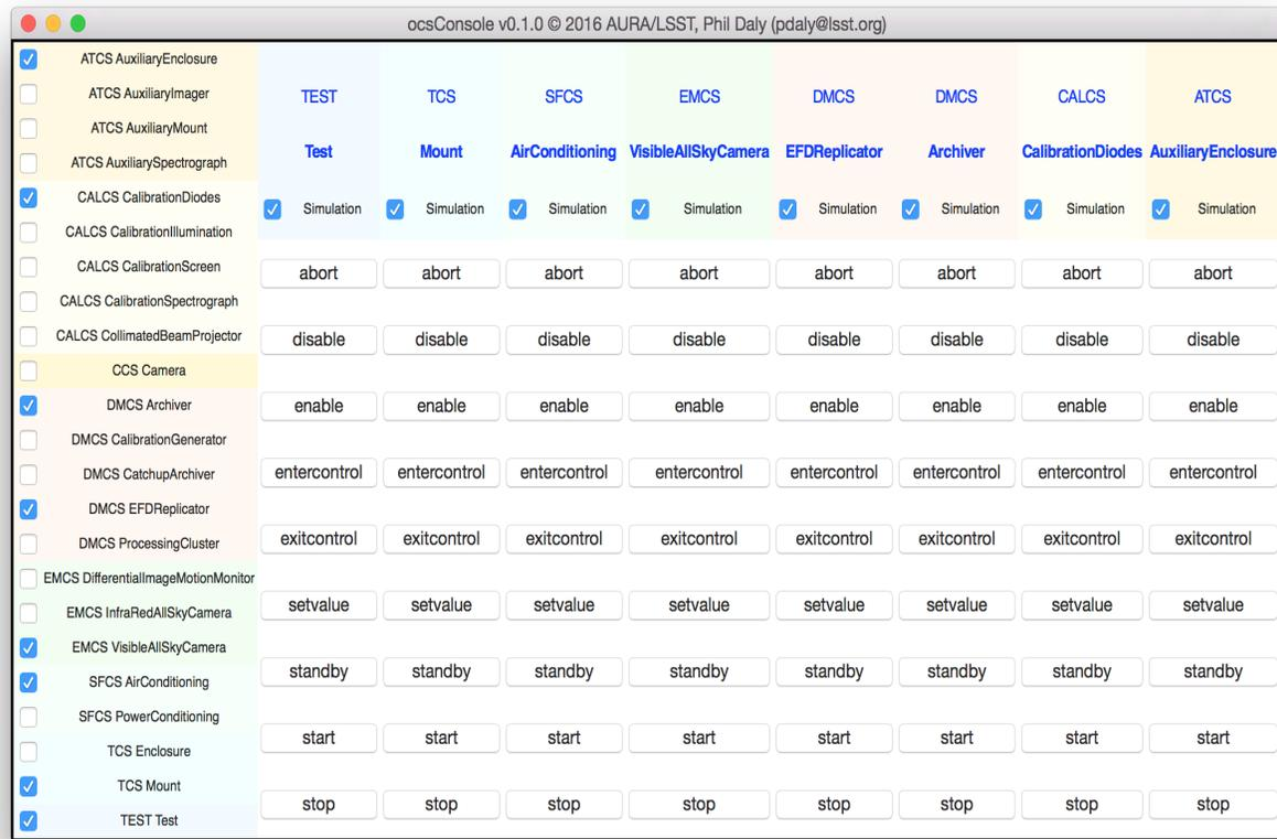
Figure 10. A tkinter console re-using sequencer classes. This is a GUI wrapper to the classes developed for the *Sequencer* and provides a dynamic OCS console.
